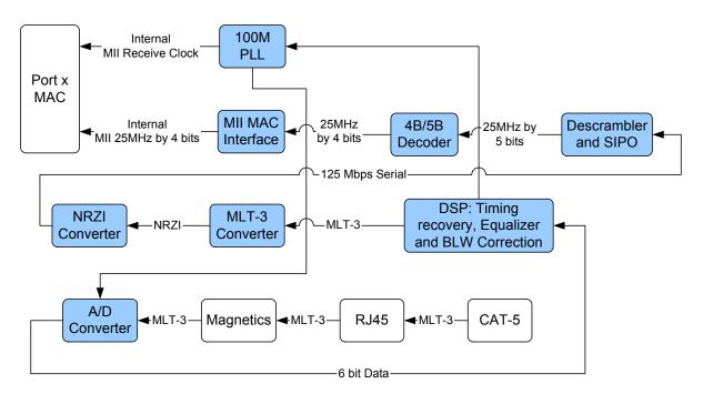
Figure 7.3 100BASE-TX Receive Data Path
