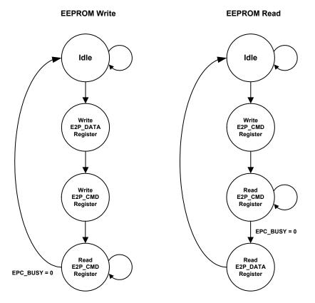
Figure 8.1 illustrates the process required to perform an EEPROM read or write operation.
