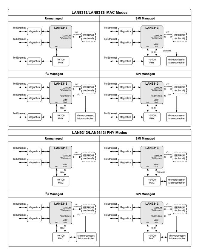
Figure 2.2 System Block Diagrams - MAC/PHY Modes of Operation
