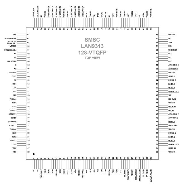
Figure 3.1 LAN9313 128-VTQFP Pin Assignments (TOP VIEW)
