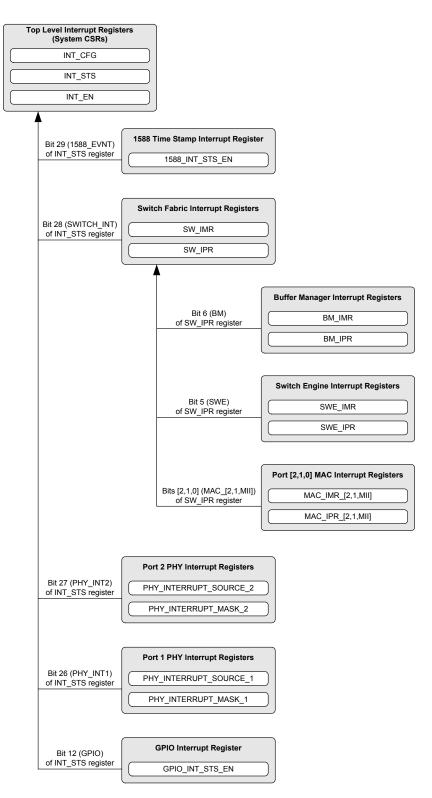
Figure 5.1 Functional Interrupt Register Hierarchy
