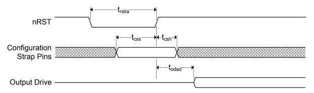
Figure 14.2 nRST Reset Pin Timing
