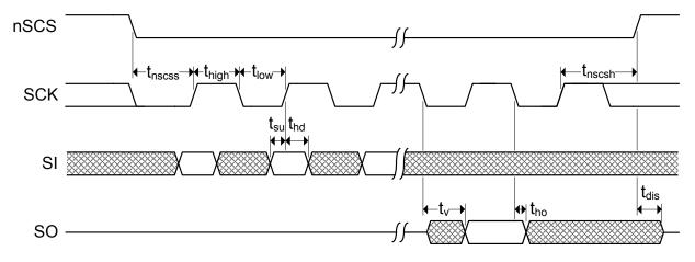
Figure 14.5 SPI Slave Timing
