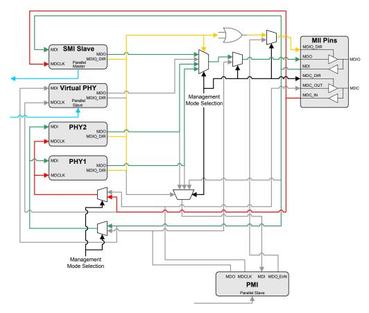
Figure 9.2 MII Mux Management Path Connections - MAC Mode SMI Managed
