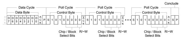
Figure 8.6 I<sup>2</sup>C EEPROM Byte Write
