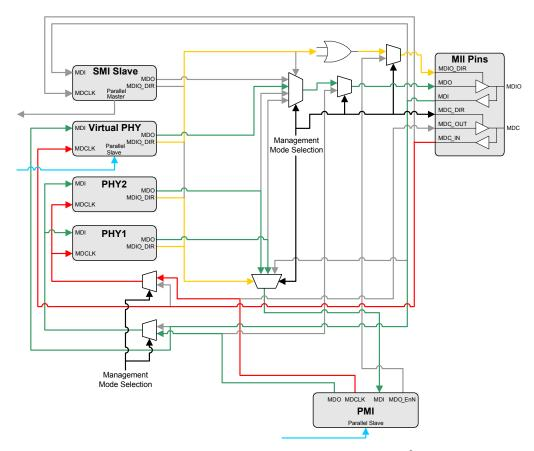
Figure 9.6 MII Mux Management Path Connections - PHY Mode I<sup>2</sup>C/SPI Managed
