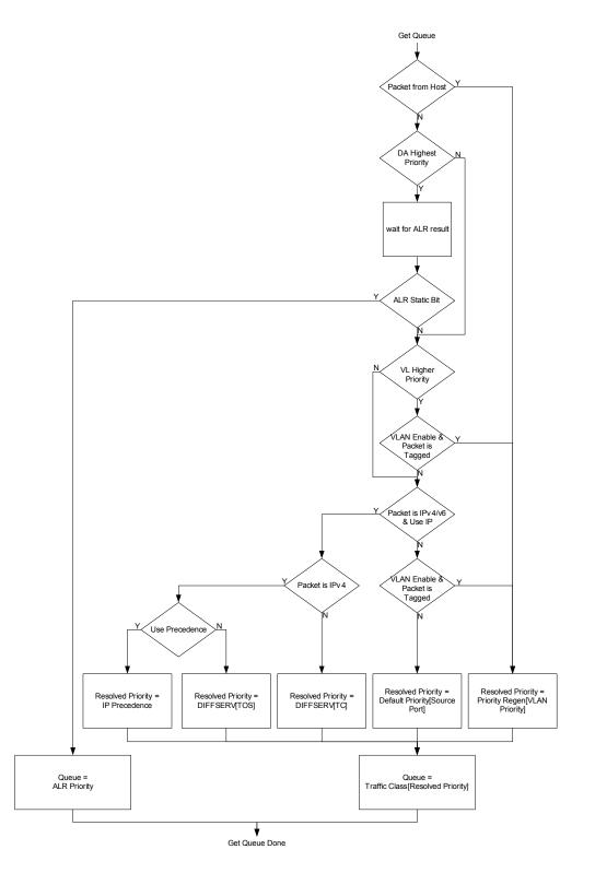
Figure 6.5 Switch Engine Transmit Queue Calculation
