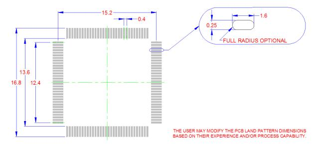
Figure 15.2 128-VTQFP Recommended PCB Land Pattern
