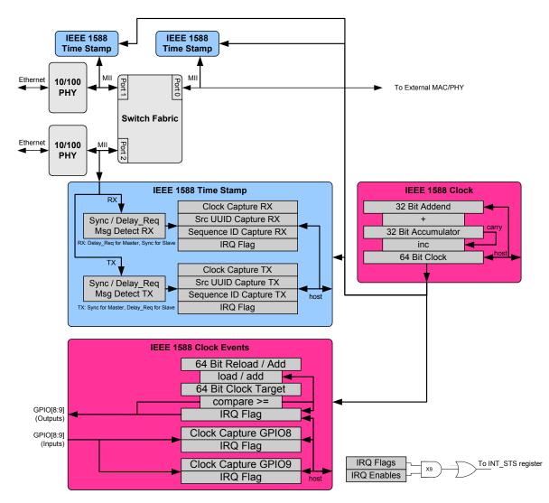
Figure 10.1 IEEE 1588 Block Diagram
