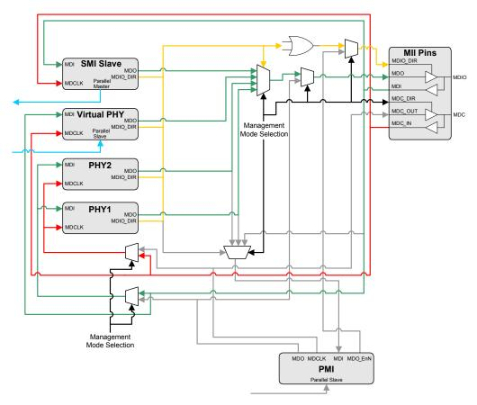
Figure 9.5 MII Mux Management Path Connections - PHY Mode SMI Managed
