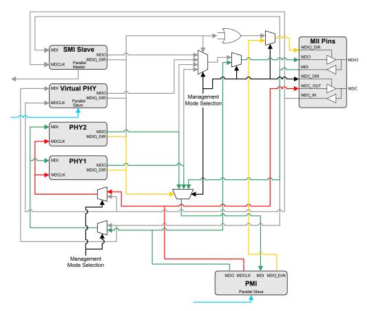
Figure 9.3 MII Mux Management Path Connections - MAC Mode I<sup>2</sup>C/SPI Managed
