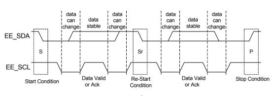
Figure 8.2 displays the various bus states of a typical  $I^2C$  cycle.
