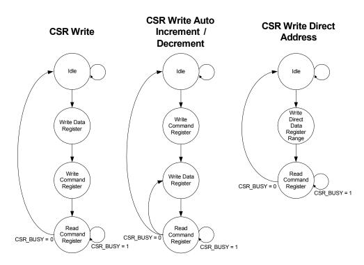
Figure 6.1 Switch Fabric CSR Write Access Flow Diagram
