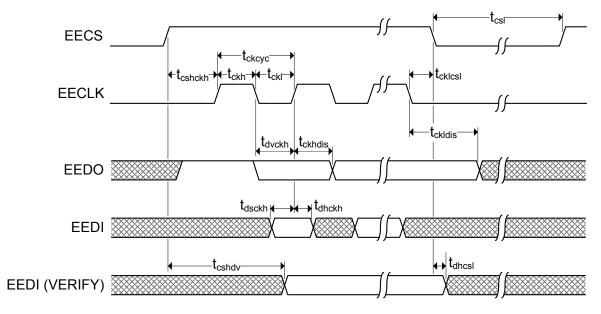
Figure 14.4 Microwire Timing
