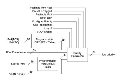
Figure 6.7 Switch Engine Ingress Flow Priority Selection
