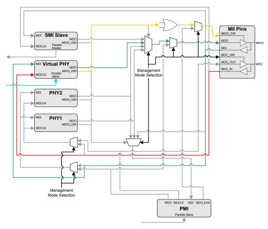
Figure 9.4 MII Mux Management Path Connections - PHY Mode Unmanaged
