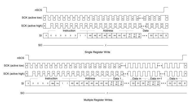
Figure 8.2 illustrates a typical single and multiple register write.
