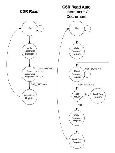
Figure 6.2 Switch Fabric CSR Read Access Flow Diagram
