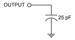
Figure 14.1 Output Equivalent Test Load
