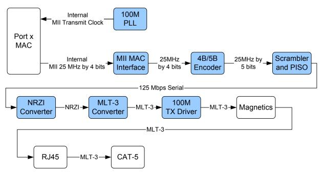
Figure 7.2 100BASE-TX Transmit Data Path
