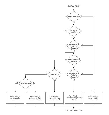
Figure 6.8 Switch Engine Ingress Flow Priority Calculation
