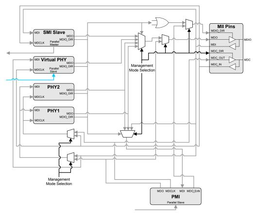
Figure 9.1 MII Mux Management Path Connections - MAC Mode Unmanaged
